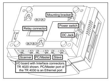
The TR40xx can be used as a wall-mount or a desktop device. You can place it on the wall using the Terminal's mounting brackets (see the Figure to the left). For desktop operation, the Terminal base can be rotated 180 degrees (to adjust the front panel's viewing angle and move away I/O connectors)- see <u>Rotating</u> base cover for desktop operation.
