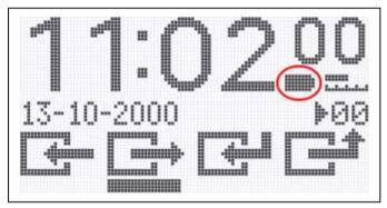
Whenever the TR40xx is running off internal battery, a Battery icon is displayed on the TR40xx screen in the <u>Normal Mode</u> (see Figure to the left). The icon can either display a "full" battery (**—**), or a "low" battery (**—**). The TR40xx will only last for about 30 minutes after the "low" battery icon is displayed.
