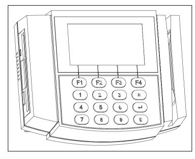
The TR4020 and TR4030 are Online Time Recorders with built-in Floppy Disk Drive. The difference between the two models is in the online interface: the TR4020 utilizes an RS232 communications network, while the TR4030 has an Ethernet port and can be placed on the Local Area Network (LAN) directly.
