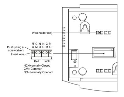
The TR40xx features two identical internal Relays with 2A switching capability (average current, peak current can be up to 10A). Relay #1 is used to control an external Bell (Ring), relay #2 controls an Electric Lock. Both normally-closed and normally-opened contacts are provided.
