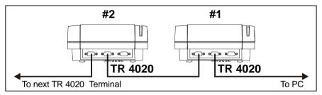
The TR4020 supports online communications via two serial ports: PC/Master and Slave. The TR4020 Terminals are interconnected in a so-called daisy-chain
