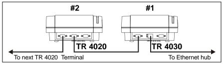
The TR4030 has a built-in UTP Ethernet port so it can be placed on the Local Area Network (LAN) directly. Each TR4030 must be assigned a unique IP address that is not
